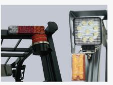
The forklift is equipped with standard LED lamps: headlamps, front turn lamps, rear combination lamps, warning lamps. Bright light with low power consumption allows you to operate freely at night.
