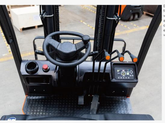
Ergonomics design for comfort operation with wide mast view and easy right-sided control levers and easy steering wheel with knob.
