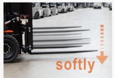
Intelligent buffering when descending to the ground, effectively protecting the ground and cargo from damage.
