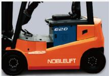
The vehicle hood and the left and right small side- panels are formed by steel plates at one time, which is simple and decent and more convenient to operate.
