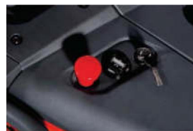
Key-switch, emergency switch and battery discharge indicator.
